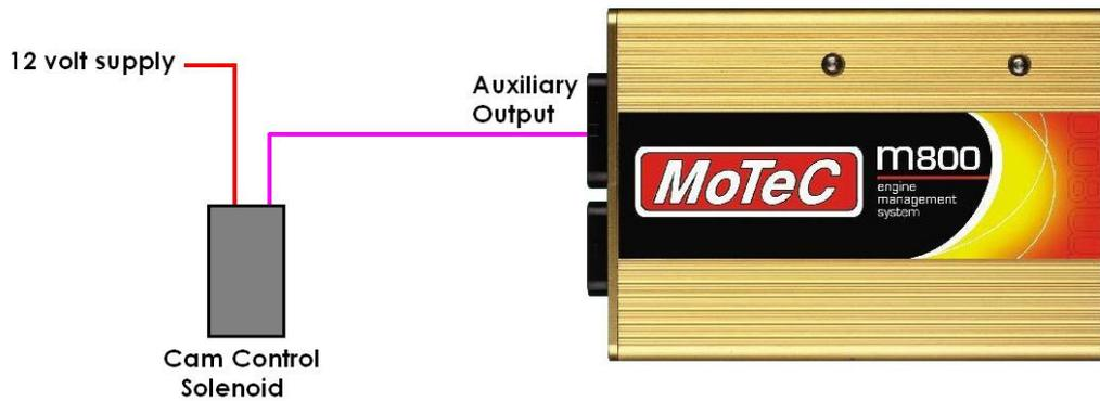
The default setting **0 : 100% duty = output low** is used when the duty cycle needs to increase to advance the cam (cam position gets larger).
