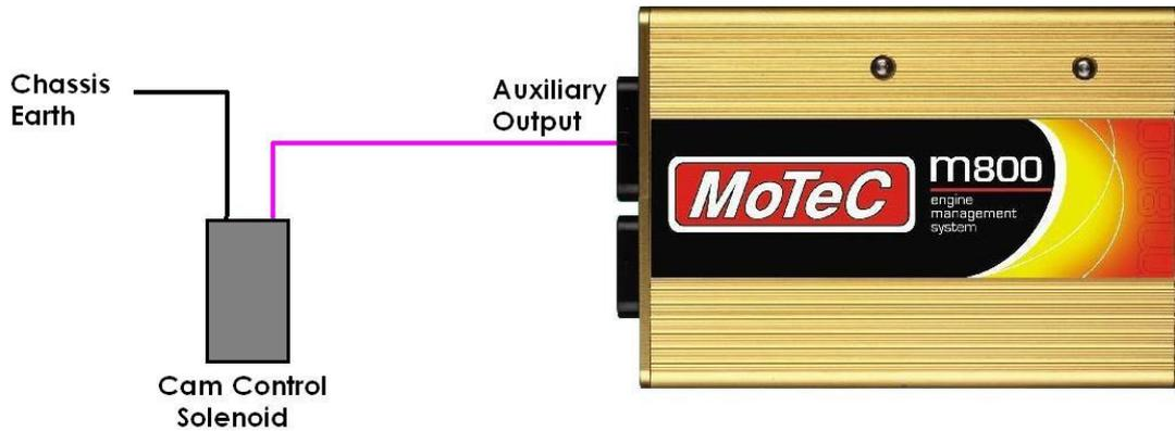
The same method can be used to decide the correct polarity for the control of a particular cam, only in step 4 the Output Mode in the parameters for the Auxiliary table should be set to **1: High Side**
