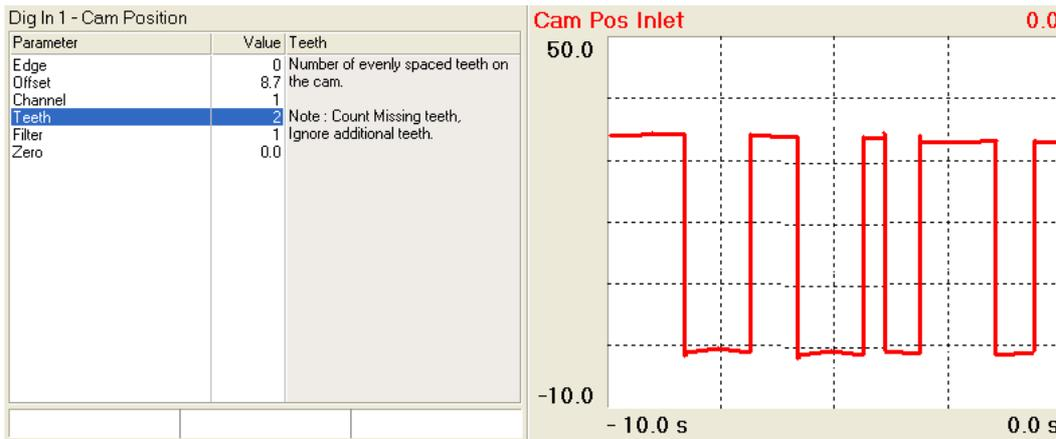
Some current factory cam position tooth patterns can be difficult to work out the number of even teeth, as a simple test the tuner could cycle through the Teeth setting numbers until a smooth cam position measurement is found. It is recommended that this only be done with the cam solenoid unplugged to ensure the ECU does not try to control the cam with an incorrect setting, this could lead to confusion as the cam position jumps around due to an incomplete setup.
