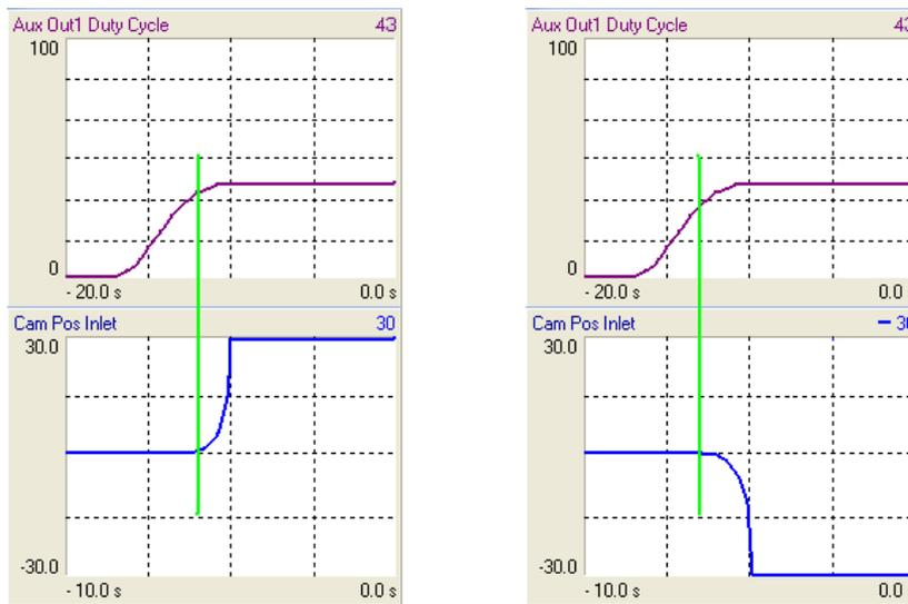
In both these examples the cam starts to move at approximately 40% Duty Cycle but the left one advances (increasing cam position) while the other retards.
