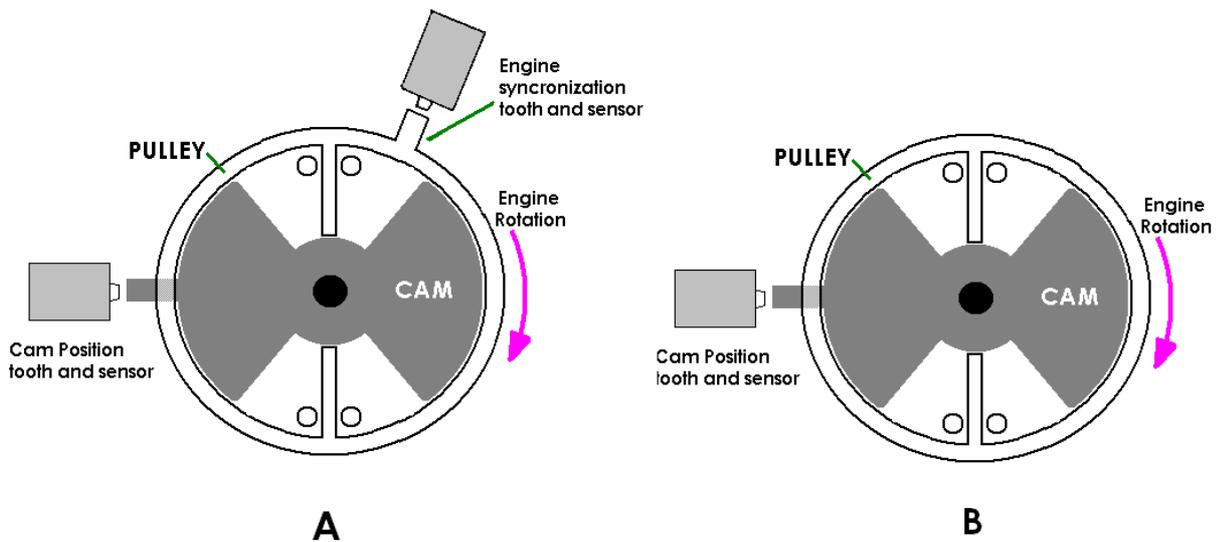
**Note:** The above diagram is a simplified example; a single tooth for each situation is extremely uncommon. Normally the combination of the crank and cam triggers results in quite complex tooth patterns.
