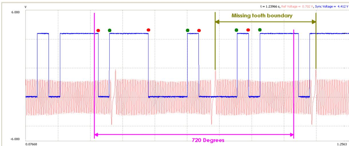
The closely spaced rising edges can be used as a synchronization point that can be referenced to the missing teeth on the crank. The ECU can calculate where the engine is in its cycle and control the injection and ignition points precisely to start and run the engine. Once the engine is running, the evenly spaced edges are used in a separate calculation to work out the cam position.
