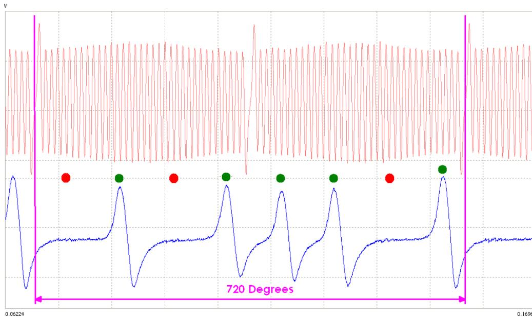
An incorrect Teeth parameter will result in an incorrect cam position calculation. With the engine running the cam position calculation will jump between two or more different positions. See the following example.
