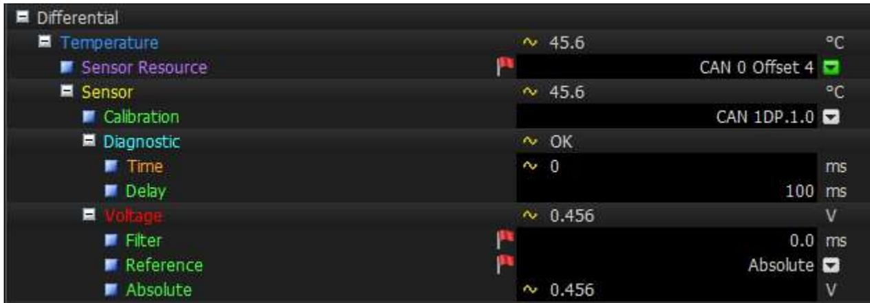
From the **Sensor Calibration** dropdown list, select the **CAN xDP** calibration option, dependent on the number of decimal places being transmitted. As the value being transmitted from the Dash is a whole number, without a decimal place, it is important to select the correct option here.
