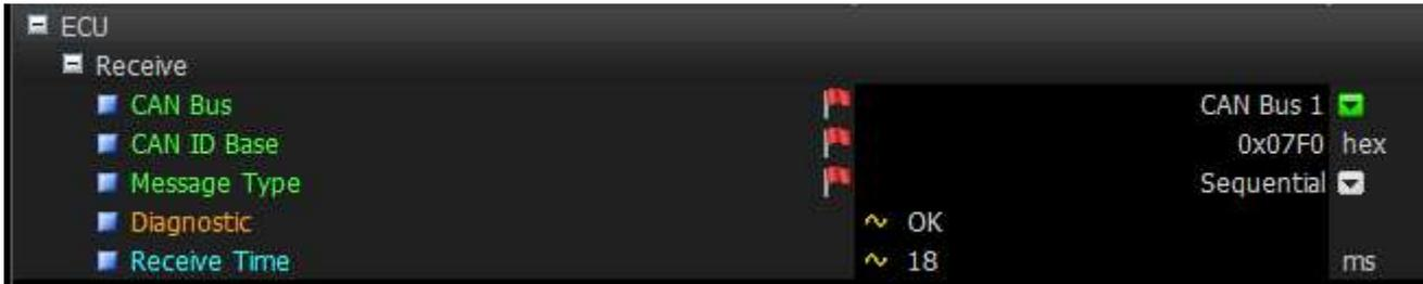
This is how the Dash **Base Address** relates to the M1 **CAN ID**, it is not possible to use a different CAN address range for some messages to the M1 to that specified as the **ECU Receive CAN ID Base**. The offset in the Dash matches that of the M1.
