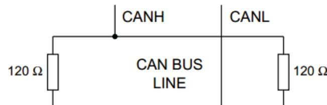
Each end of the CAN bus is terminated with 120Ω resistors in compliance with the standard to minimize signal reflections on the bus. You may need to place a 120Ω resistor between CAN-L and CAN-H.
